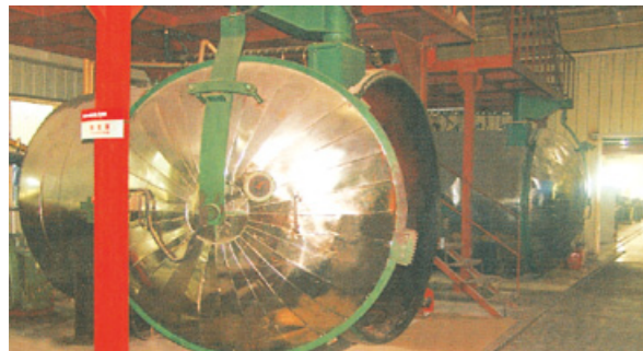
真空浇注设备 Vacuum casting equipment
