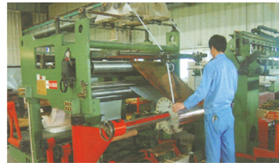
箔式绕线机 Foil winding machine
