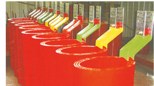
低压箔式线圈 LV foil winding
